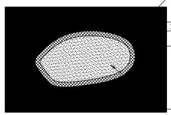
DEFECTIVE PAVEMENT - POTHOLE, BIRDBATH, OR ALLIGATORING
